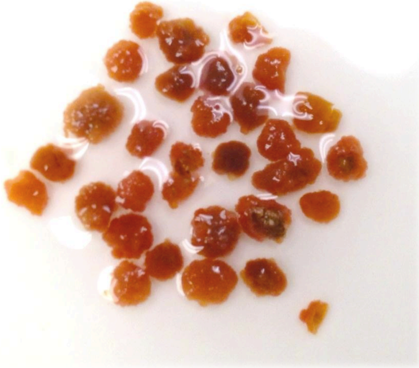
Fig. 7 Granules in UASB Anammox reactor (diameter approximately 3 mm)
